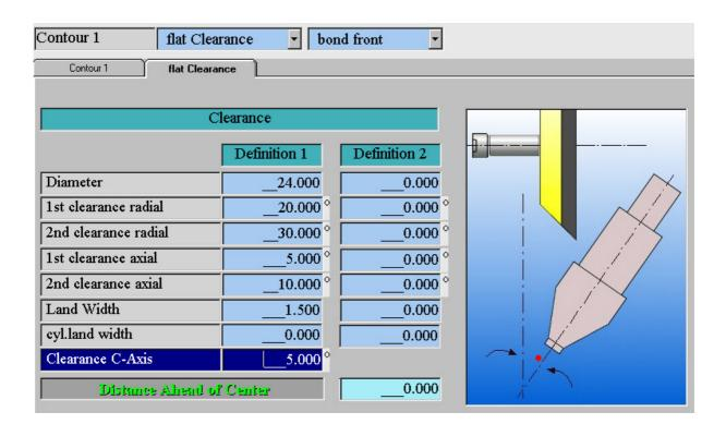
Front teeth can be probed "ahead of center". It can be grinded with all grinding methods.
