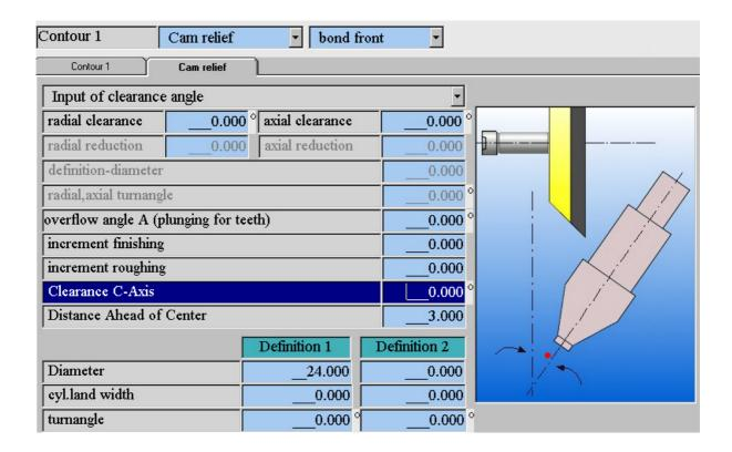
New grinding method "flat clearance" – the clearances are not grinded with hollow grind. They are grinded with the front bond of the wheel.
