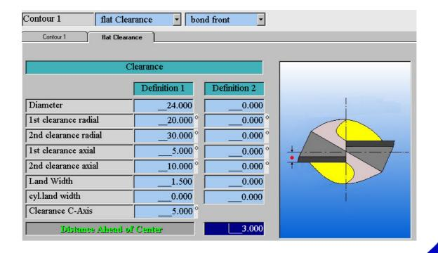
New grinding method "front teeth ahead of center with negative chamfer" The 1. clearance will be grinded negative. The cutting edge will be generated at the transition of 1. and 2. clerance.
